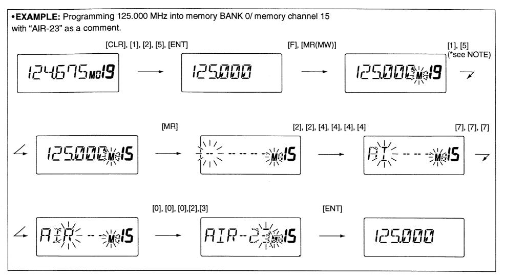
\*NOTE: Push [BANK], then rotate the [DIAL] to select the BANK number, if desired. Push [CLR] to continue memory name programming.
